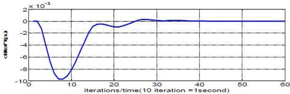
Figure 6: change in frequency V/S time in area-1 for 0.01 step load change in area-1
