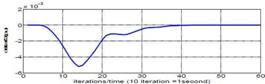
Figure 7: change in frequency V/S time in area-2 for 0.01 step load change in area-1
