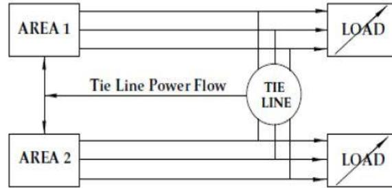
Figure 1: Two area interconnected power system
