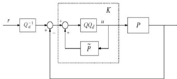
Figure 4: IMC equivalent conventional feedback configuration
