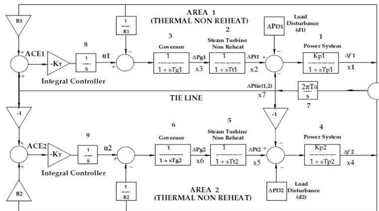
Figure 2: Two area thermal (non-reheat) power system with integral controller
