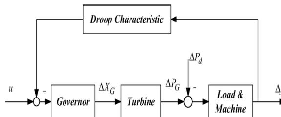
Figure 5: Linear model of a single area power system
