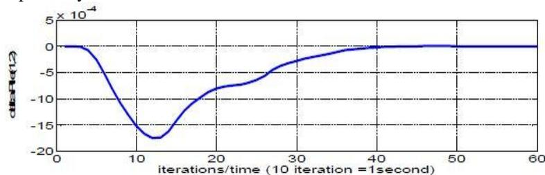
Figure 8: change in tie line power V/S time for 0.01 step load change in area-1
